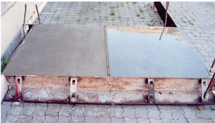
Image 1: trial slab, on the left without AF, on the right with AF
